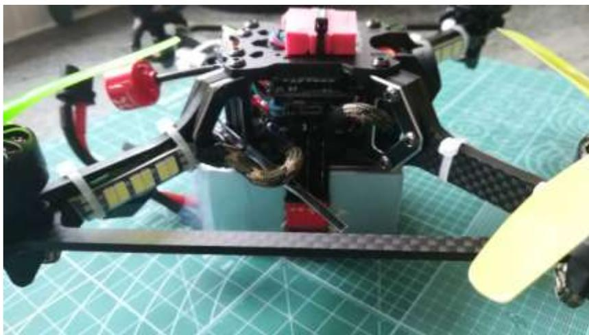
and now, 4 new motors. All I needed was a video transmitter (VTX) and I set about this new build. In hindsight I should have documented the build because it was just as challenging as the B test build will be. It took about a week to finish and once completed I decided to add a GPS and 3d printed a holder for it. The camera has the ability to record 1080p HD video and has a micro SD card slot for the recording of video.
