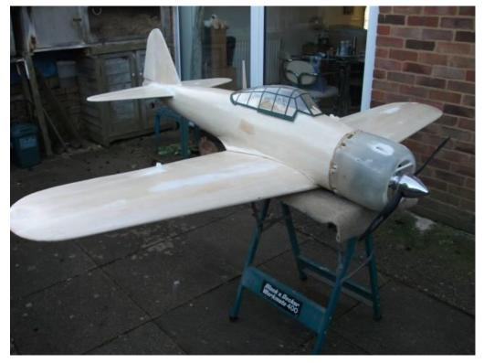
rewarding. At 92" span and slightly larger than 1/5 scale it's a large model. The tailplane spans 38" which means it will only just go in the Mondeo. I still have some minor fettling to do but I now have two large lumps, i.e. the fuselage complete with rear
