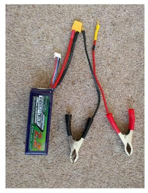
. This is what I came up with. A 3 cell 2.2AHr lipo battery and crocodile clips. The engine span like a dervish and fired instantly. Once running I removed the lipo and drove off to Halfords. The lipo came with me in case I stalled the car. The young fitter who changed the duff battery couldn't believe that I had started the car from such a small battery.
