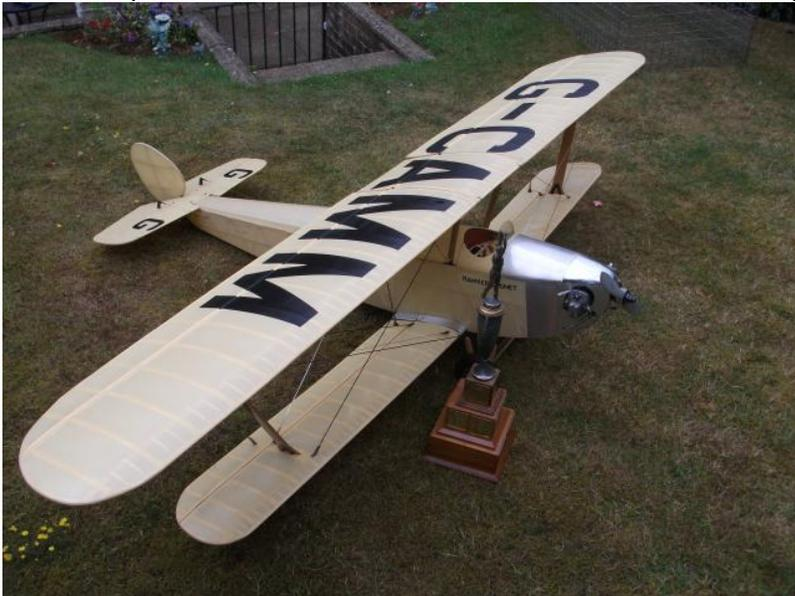
Sunday. The landing area at OW is not particularly flat and the grass really grabs small wheels. My lower port wing suffered slight damage which I superglued on the spot but I have now done a proper repair which entailed removing the wing and recovering two rib bays. This is fairly easy to disguise
