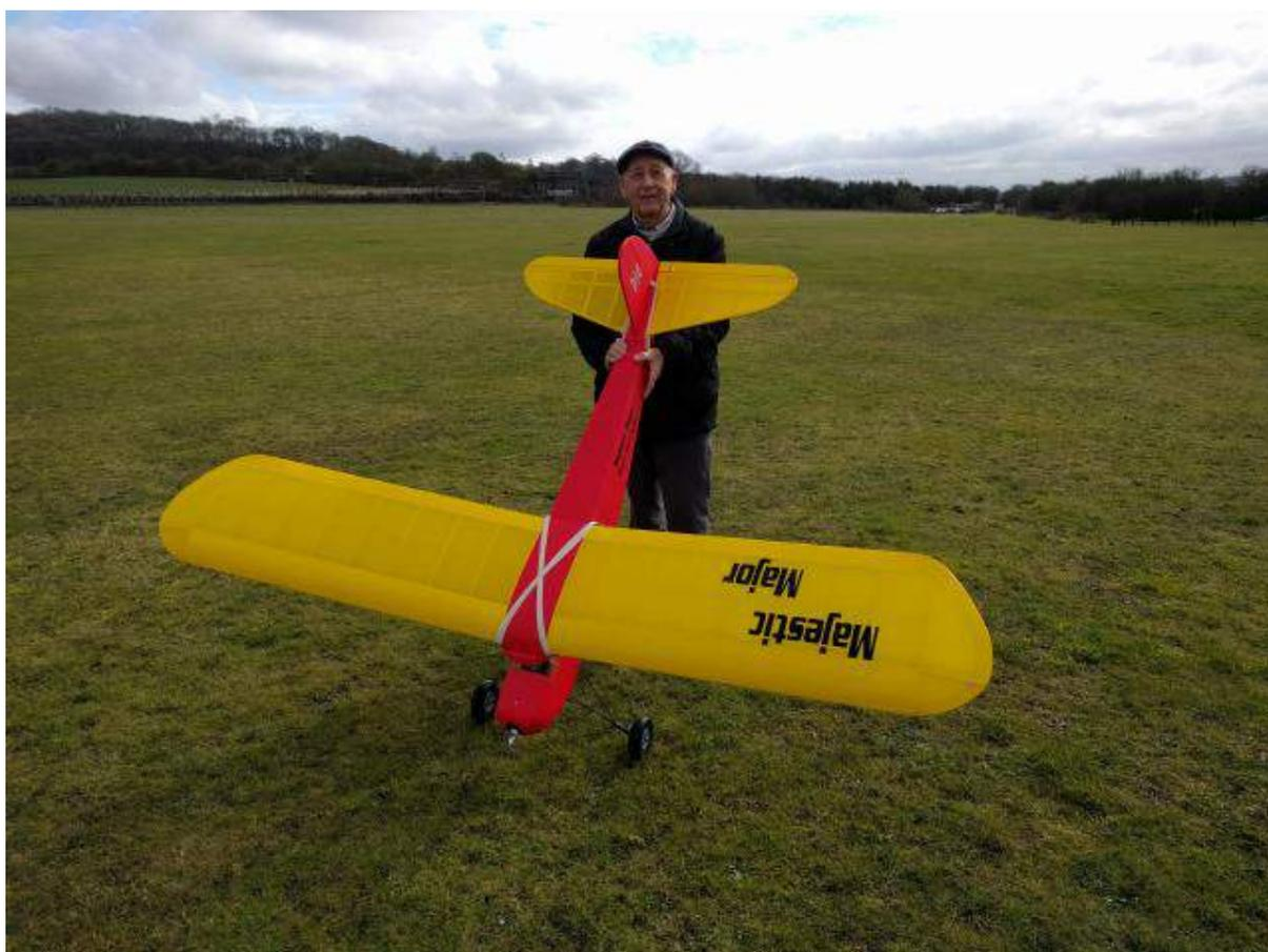
During the winter I decided to build a Ben Buckle Majestic Major. I intended to eventually fit a 70 Four Stroke glow after initially electrifying it. The Tornado Thumper is mounted on a bracket onto the beech bearers. The 4s 4500 Lipo easily fits in and without much modification all could be removed to go glow.
