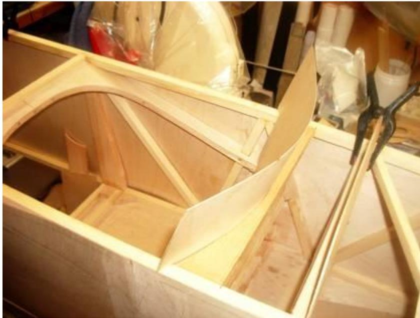
**With the back temporarily in place the curvature of the turtle deck was scribed in before cutting it to shape and gluing in place – more clamps!**
