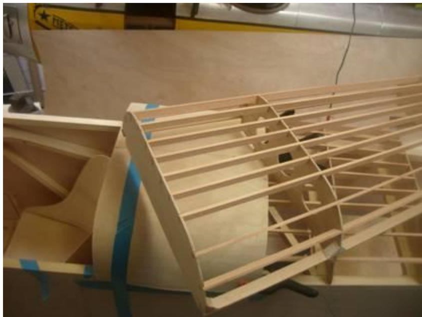
**The centre section of the turtle deck was made removable in order to access the electronics. Just four bolts hold it in place.**
