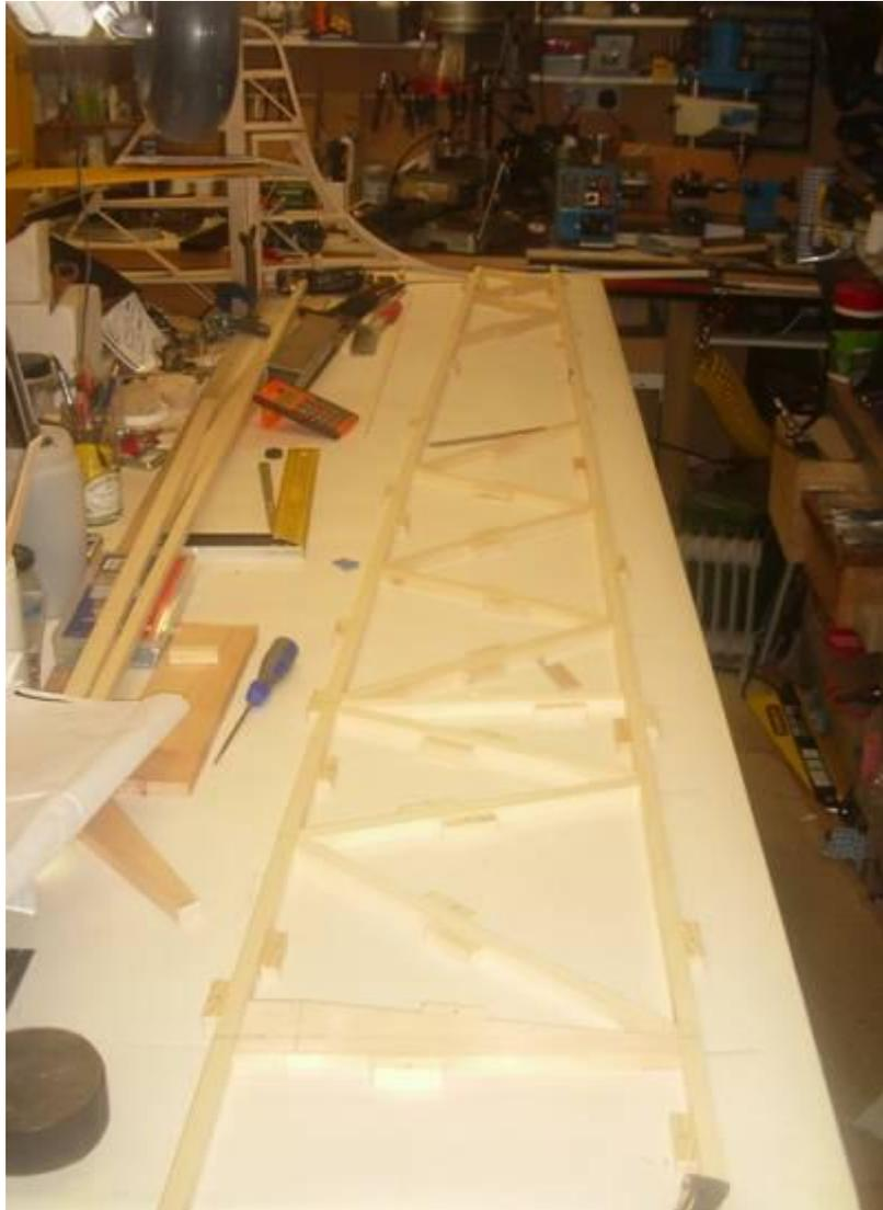
**All the components in place for a final check on the fit before the gluing was started.**
