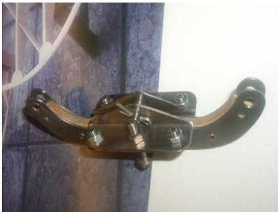
**One of the more complex pieces – the elevator control horn and central elevator hinge. sandwich construction for stiffness**
