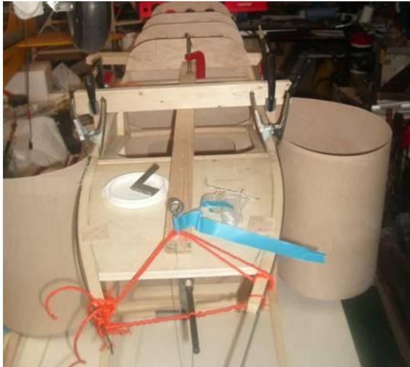
**Steam, string and clamps eventually had the longerons in the front end of the fuselage bent to the correct curvature. Note the ply sides folded back out of the way ready to be glued in place after the longerons were secured.**
