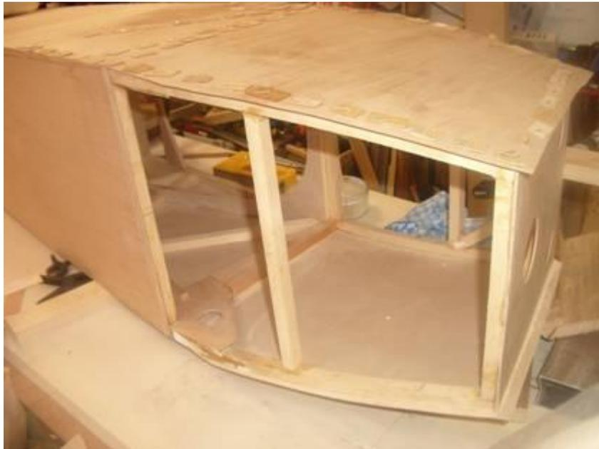
**With firewall in place the sheeting of the underside was finally attached, same procedure – Cascamite and many many staples**
