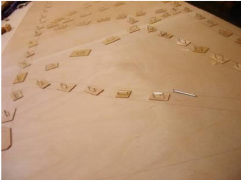
**Same technique used to glue the sheeting to the fuselage sides: Cascamite this time to give more time to complete the stapling**
