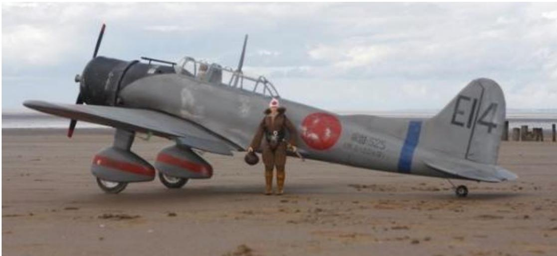
This is a Chris Willis design, 84 inch span and has a fixed u/c. Definitely a "builder's" project, I have seen Chris's own model (at the Bickley scale meet) and picked up a few tips. His flew on a 90 two stroke, unfortunately I can't get a four stroke in the short cowl so have bought another 120AX, the same motor as fitted to the big FWTA152 so I will certainly have bags of power!
