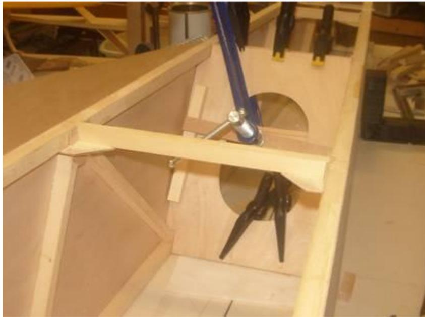
**Having fitted the gussets in place the bottom of the fuselage was sheeted and the first of the bulkheads fitted**
