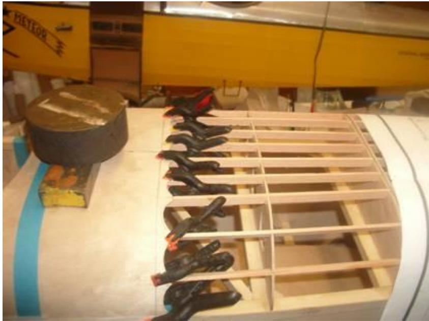
**Stringers glued into their slots and the short ply deck aft of the cockpit being glued into position. More clamps!**
