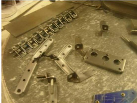
**Hinges; tailplane attachment plates cleaned up and ready for plating**
