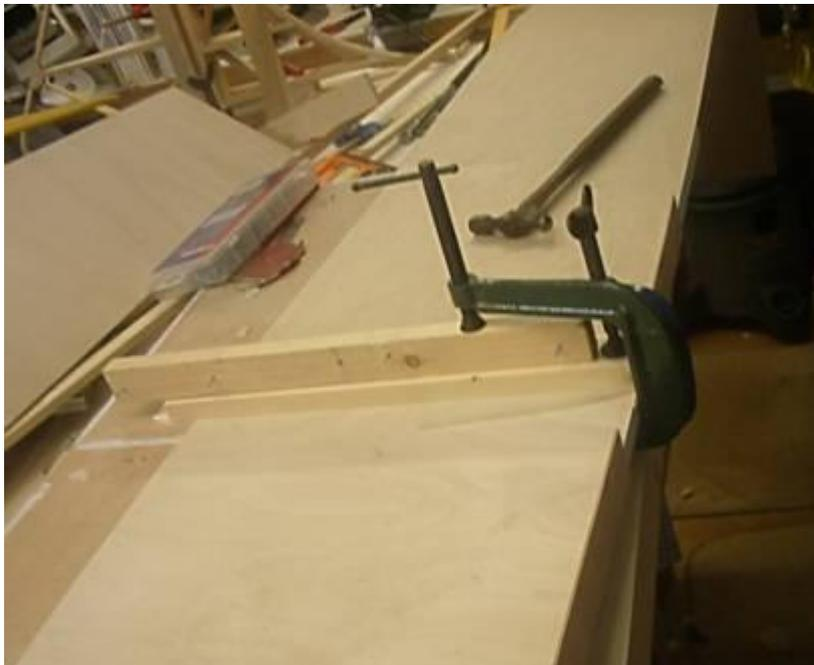
**Once the scarfs were roughed out on my scarfing rig they needed a bit of fine tuning before they could be glued together**
