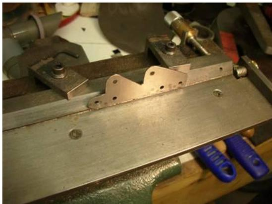
Having punched the holes and set up the bend allowance the first bend was made
