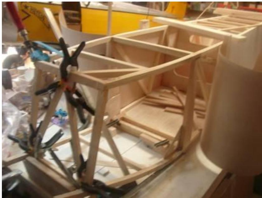
**Securing the longerons and framing the firewall.**
