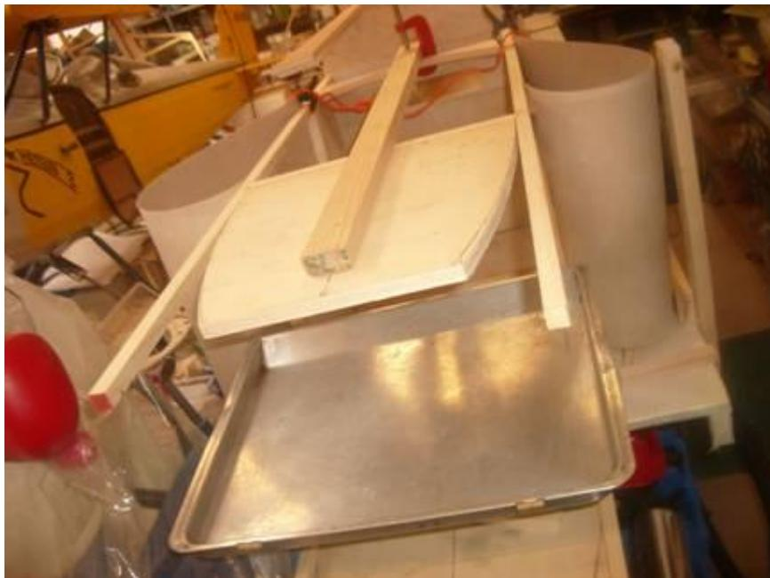
**Setup ready to soak the longerons prior to bending**
