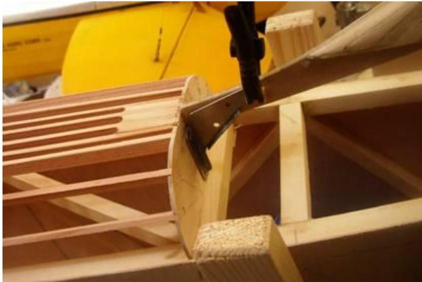
*Checking the fit of the fin and its metal fitting at the tail end.*
