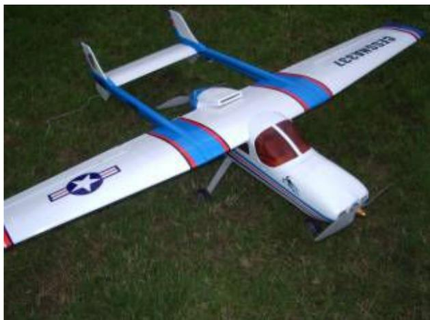
suppliers for one, and ended up importing it from Hong Kong. The model is a Cessna 337 and is an ARTF in all built up balsa and ply. With a 1.55m wingspan, there are two motors, in line, one tractor and one pusher. Originally designed for 0.25 ic engines, I have put in two 400W brushless motors running off a 4 cell lipo.
