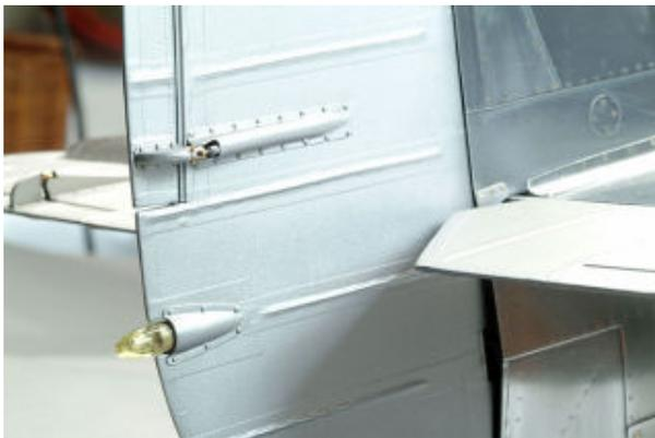
*The model is skinned with litho plate over a balsa core and has been left in bare metal at the suggestion of Michael Fopp, so that the structure is seen to best advantage. The rivets are real and many are pushed into drilled holes in the skin and underlying balsa, but many more are actual mechanical fixings. I have no*
