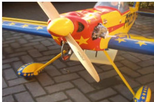
As you can see the engine is now installed in my 120" Eurobat. Originally with 80cc boxer the model weighed 35lbs. Approx, now with the 120cc it only weighs 36.5lbs and it hasn't got the 4lb of nose weight that it had before, things are looking very promising, I digress.
