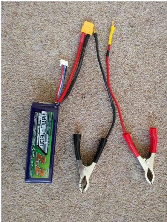
. This is what I came up with. A 3 cell 2.2Ahr lipo battery and crocodile clips. The engine span like a dervish and fired instantly. Once running I removed the lipo and drove off to Halfords. The lipo came with me in case I stalled the car. The young fitter who changed the duff battery couldn't believe that I had started the car from such a small battery.
