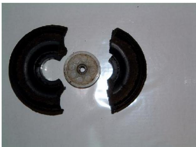
Lastly, one check I've never thought of making before are the tyres. The reason for mentioning this is just recently I suffered an unusual experience. I was preparing to take off with my Sbach, full throttle and at the point of rotation the plane stopped dead and nosed over with an almighty thump. First thoughts were I'd dropped a
