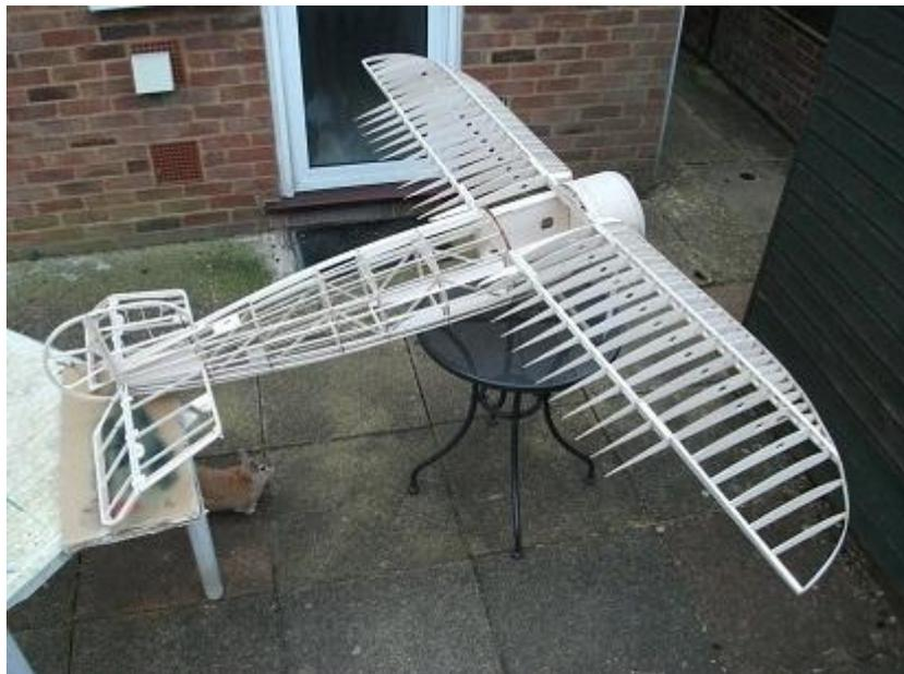
has to be practical, reliable and fairly easy to rig and fly so I have made some compromises with the ailerons and rigging. The whole structure aft of the wing leading edge is built up, much like my Morane A1. Span is 92" and quoted weight is 15lbs. I have chosen a Laser 180 engine running an SM Services on board glow for starting convenience and tickover. There is no doubt that the Laser is the BEST four stroke
