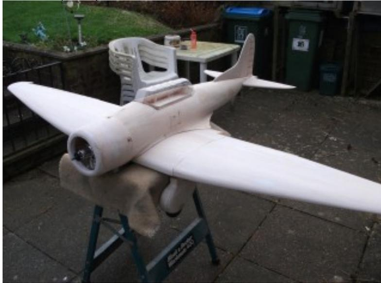
Some nose weight will be required and I plan to fit this inside the front of the cowl where the effect will be greatest. A brass spinner nut will also help, these are really useful and weigh around 2.5 ounces.
