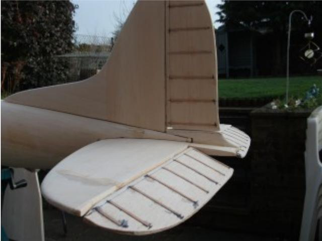
The "winter" project is nearing completion - the woodwork is finished. This morning (Friday 11 Jan) I assembled the whole lot outside on the patio. However, parts have been trial fitted along the way so there were no nasty surprises! It is
