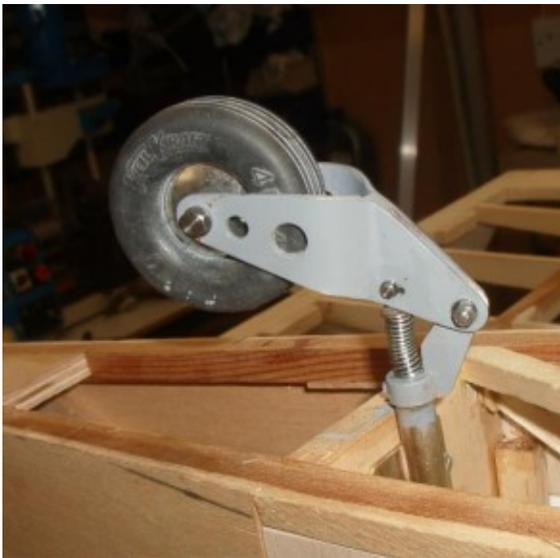
A particular and recent case in point concerned the tail wheel assembly. Most of the full sized planes built just before and immediately after the second World War used a fully castoring tail wheel pivoted on a leaf spring bolted to the underside of the tail end of the fuselage. Not such a good idea if you wanted to fly the model from a small field like ours in Newground
