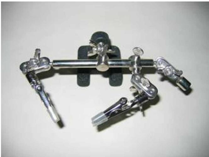
These can be purchased quite cheaply from companies like Proops Brothers, Maplin Electronics etc and comprise a heavy metal base supporting a number of articulating arms with crocodile clips on the ends, which can be adjusted and clamped in a multitude of positions. These can be used to support one or both components during soldering
