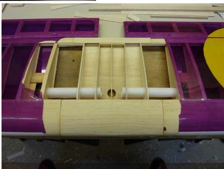
The new centre section was built and lined up for a splice on to the outer panels. With the bits joined up it was on with the dowels, top sheeting and nylon bolts
