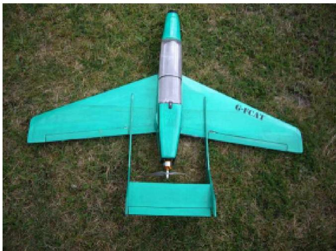
allow more air flow through the fan but there was no improvement. I then modified the fuselage to convert to a brushless inrunner driving a prop. Excellent performance but it all got too hot and the ESC gave up. The final version is fitted with a 2200kv brushless outrunner on the back end and a 6x4
