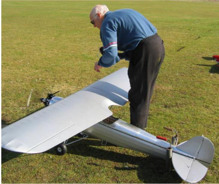
The undercarriage replicates full size and incorporates telescopic suspension with the damping supplied by several "O" rings on each leg. Big airwheels (Dubro) provide more cushioning. At this size and weight the U/C has to work and withstand the shocks of lumps and bumps and the inevitable less
