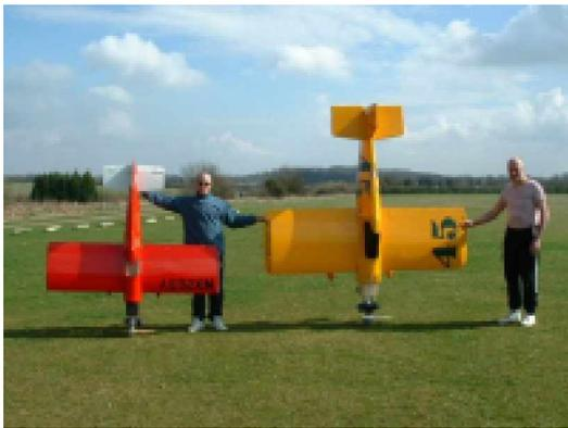
The new Cassutt weighs in at 28lbs and has a Zenoah 80 cc twin cylinder boxer motor. This was built using the same plan that I built the red one from. It actually started as a 1/4 scale plan which I enlarged for both the Cassutts. The build time for the larger Cassutt was approx 6 weeks. I am at present building the cowl for it, having had to make a mould using a hard foam and I
