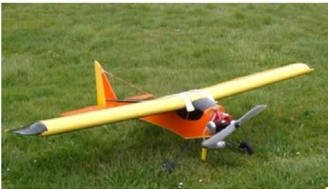
Over the following weeks, I made a new firewall and replaced all the front section of the fuselage; made a new wing seat; a new elevator, and finally got it all back together looking as good as new, before tackling the worst job: the wing.
